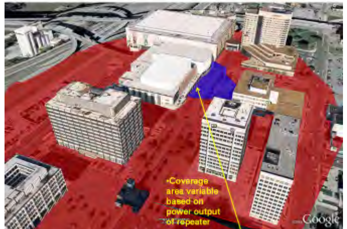
Memphis Convention Center – Body Wire w/ Repeater Coverage
